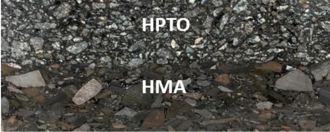
Figure 3. Thin-overlay applied to HMA.
