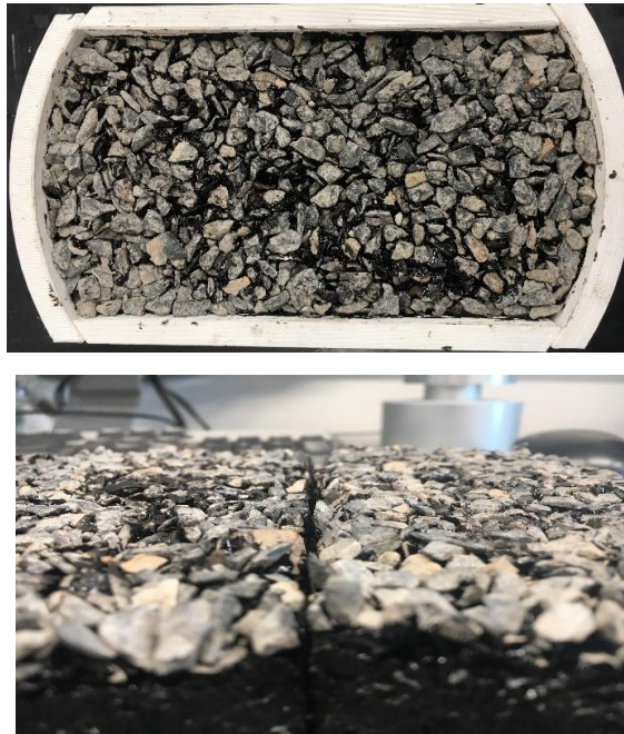
Figure 11. OT Sample with chip seal applied. A) Chip Seal in Mold B) Level Chip Seal Surface
