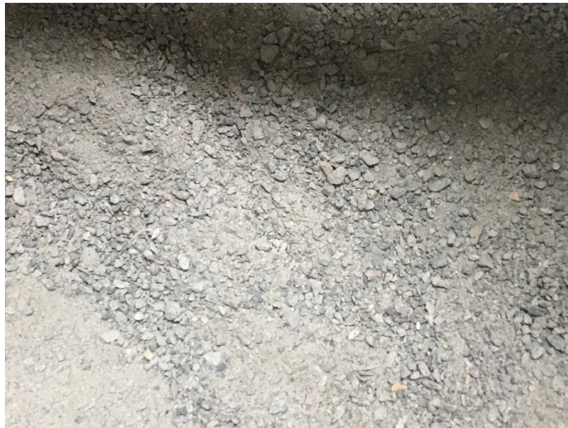
Figure 15. Type II microsurfacing aggregates (largest aggregate 9.5mm).
